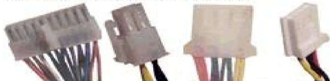
ATX 20-PIN X 1 P4 ATX 12V X 1 IDE 4-PIN X 4 Floppy 4-PIN X 2
